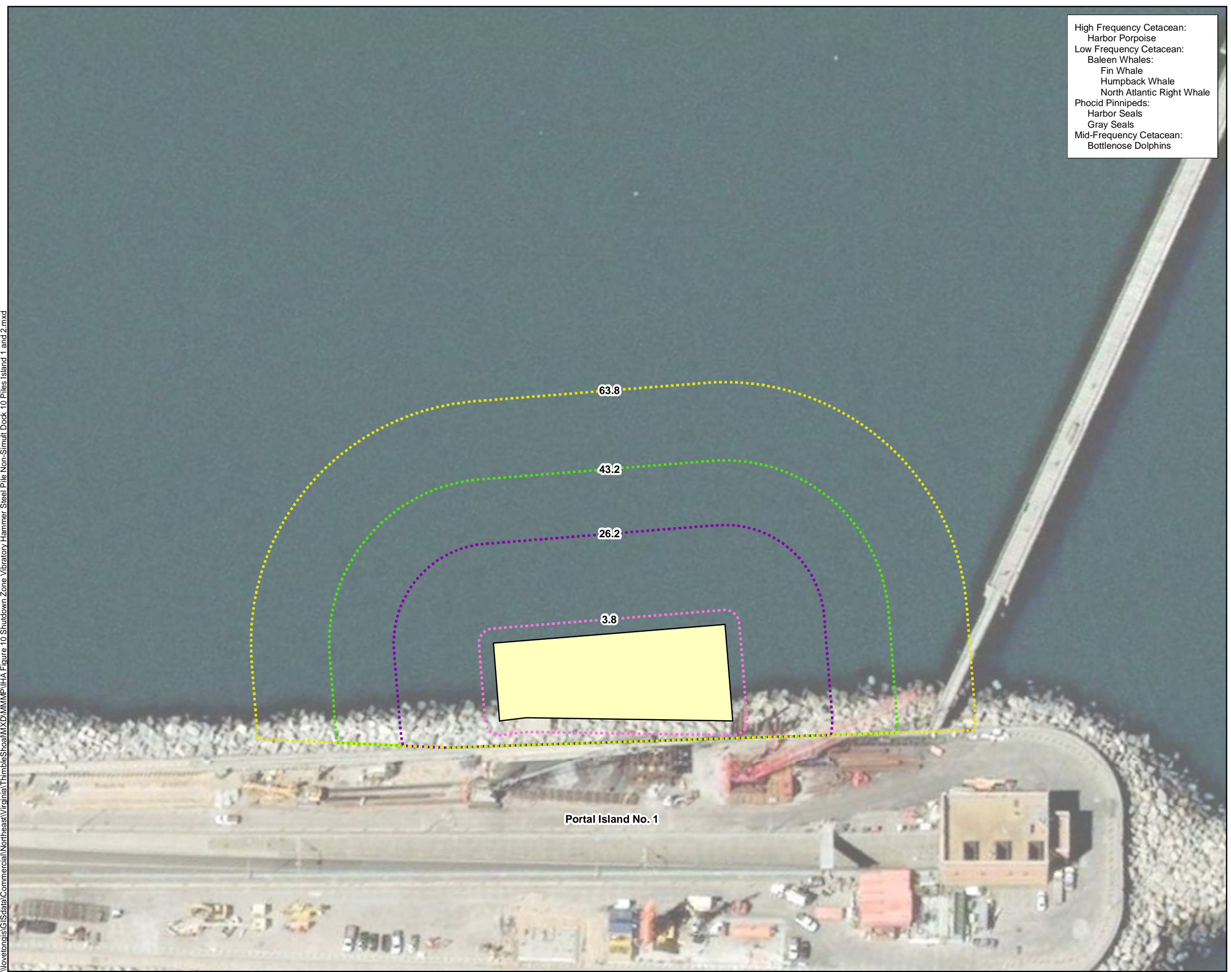
Figure 3 Distance (meters) to Shutdown Zone Using a Vibratory Hammer for Non-Simultaneous 36- and 42-in Steel Pile Driving for the Temporary Dock – 10 Piles per Day at Portal Island No. 1 Marine Mammal Protection Act Parallel Thimble Shoal Tunnel
