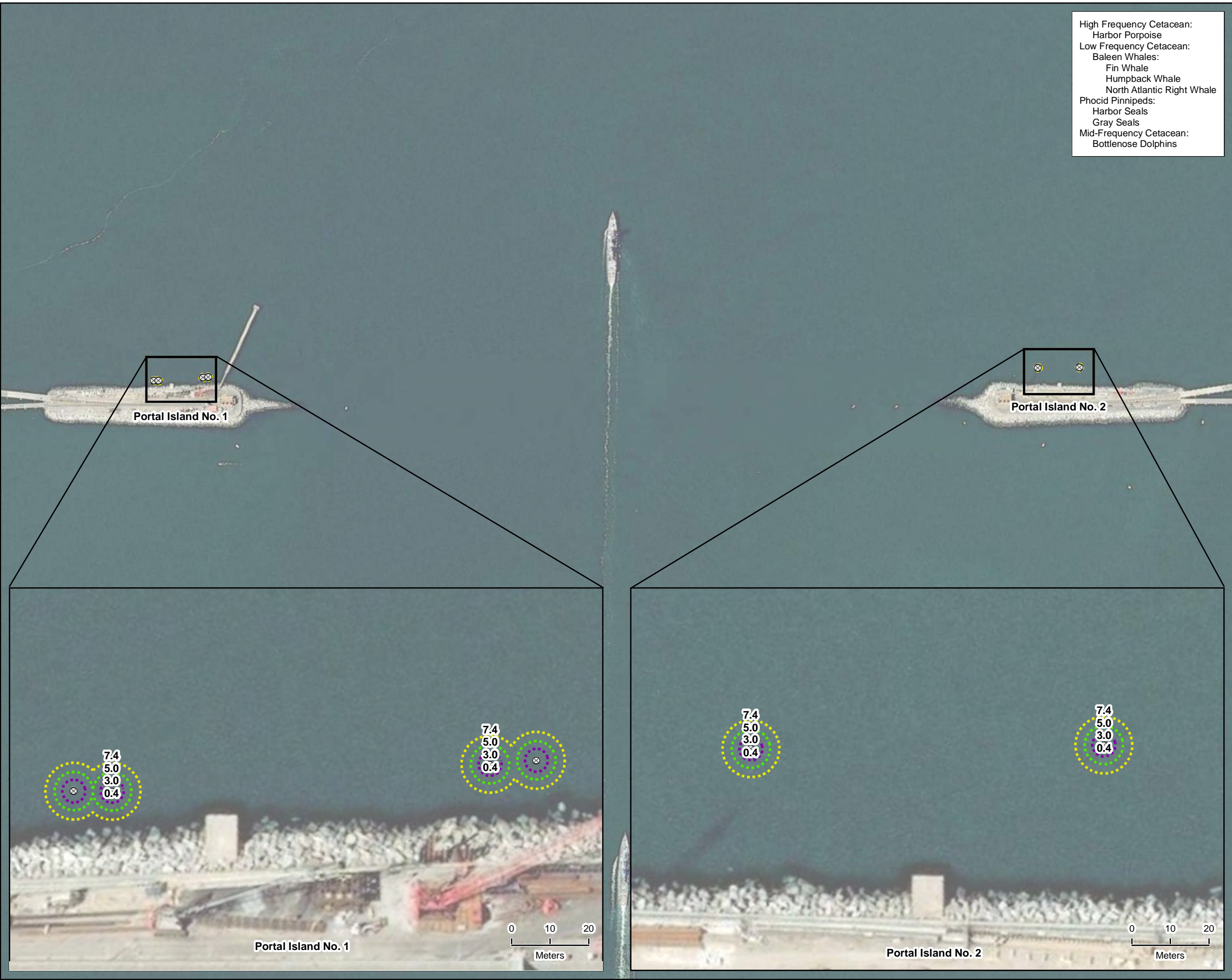
Figure 2 Distance (meters) to Shutdown Zone Using a Vibratory Hammer for Non-Simultaneous Timber Pile Driving for the Mooring Dolphins – 10 Piles per Day at Portal Island Nos. 1 and 2 Marine Mammal Protection Act Parallel Thimble Shoal Tunnel
