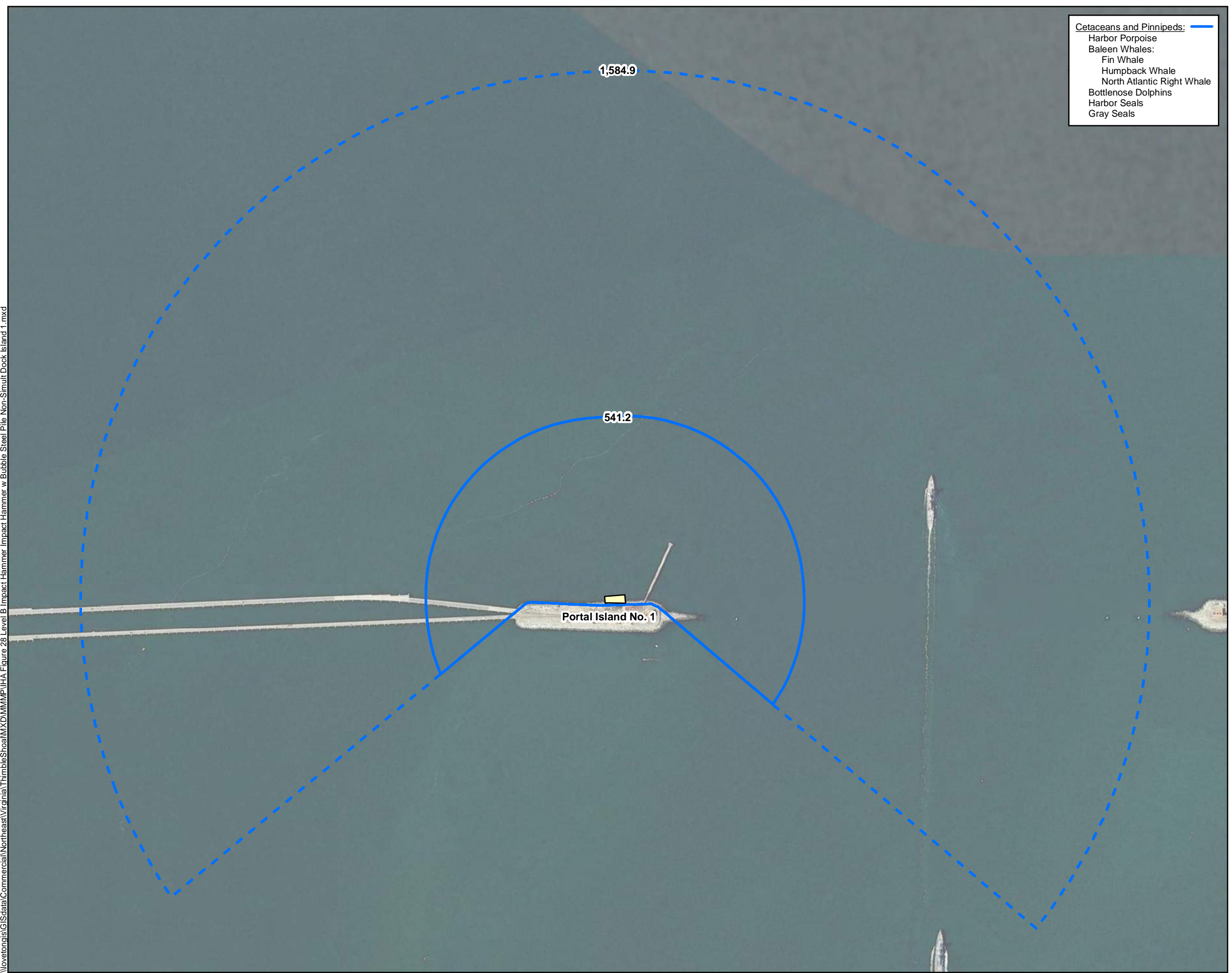
Figure 13 Distance (meters) to Level B Threshold Using an Impact Hammer or Impact Hammer with Bubble Curtain for Non-Simultaneous 36- and 42-in Steel Pile Driving for the Temporary Dock at Portal Island No. 1 Marine Mammal Protection Act Parallel Thimble Shoal Tunnel
