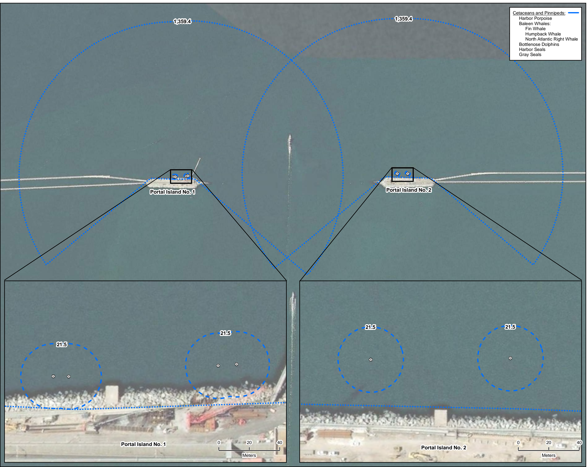
Figure 14 Distance (meters) to Level B Threshold Using an Impact Hammer or Vibratory Hammer for Non-Simultaneous Timber Pile Driving for the Mooring Dolphins at Portal Island Nos. 1 and 2 Marine Mammal Protection Act Parallel Thimble Shoal Tunnel
