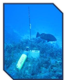
fixed locations, and can also be used to conduct video transects and census and length measurements. Together, acoustics and cameras provide a powerful combination to observe fish and fish behavior. I will present studies from two projects that have combined acoustic and camera-based methods to address research questions related to fish spawning aggregations and commercial fishing bycatch reduction devices.
