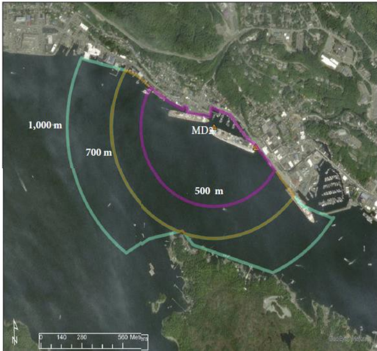
Figure 4. Level A shutdown zones for impact pile installation of 30-inch piles for 0-500 strikes (purple, 500 m), 501-1,000 strikes (yellow, 700 m), and 1,001-1,500 strikes (green, 1,000 m) at Mooring Dolphin 2 (MD-2), COK Berth III (PND Engineers 2020b).
