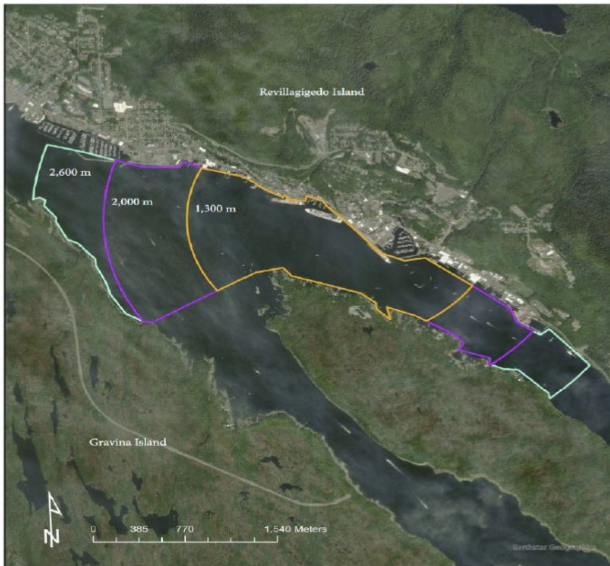
Figure 7. Level A shutdown zones for impact pile installation of 36-inch and 48-inch piles for 0-500 strikes (blue, 1,300 m), 501-1,000 strikes (purple, 2,000 m), and 1,001-1,500 strikes (yellow, 2,600 m) at Mooring Dolphins 3 and 4 (MD-3, MD-4), COK Berth III ((PND Engineers 2020b). Level A shutdown zones for DTH socketing of 30-inch and 36-inch piles for up to 3 hr (blue, 1,300 m), and 3-6 hr (purple, 2,000 m).
