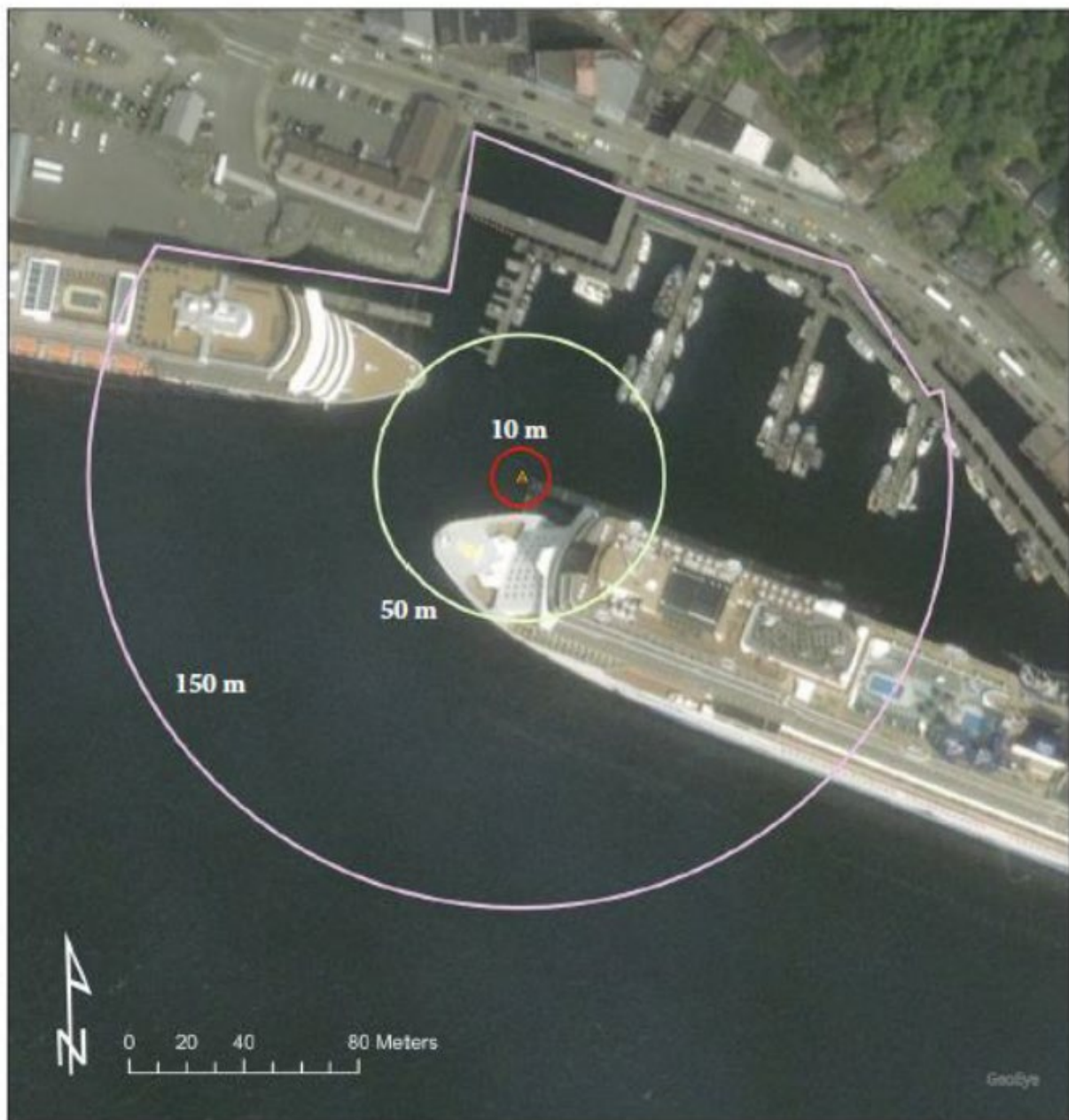
Figure 10. Level A shutdown zones for in-water or over-water non-pile driving activities (red, 10 m) and DTH anchoring up to 12-inch holes (pink, 150 m) at Mooring Dolphin 2 (MD-2), COK Berth III (PND Engineers 2020b).
