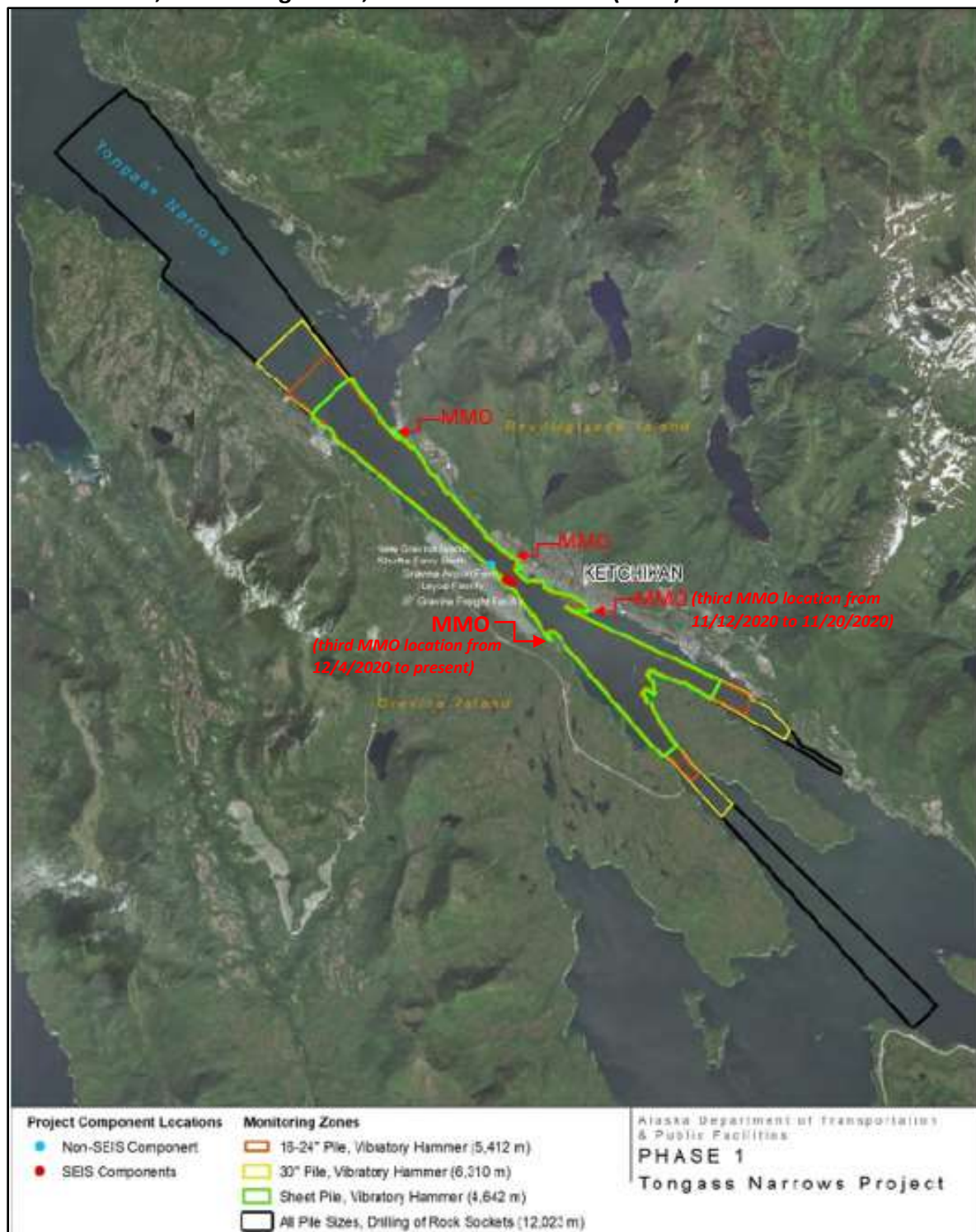
FIGURE 2. Tongass Narrows Ferry Berth Improvements: Phase 1 Construction NMFS-Approved PSO locations, Monitoring Zones, and Shutdown Zones (2020)
