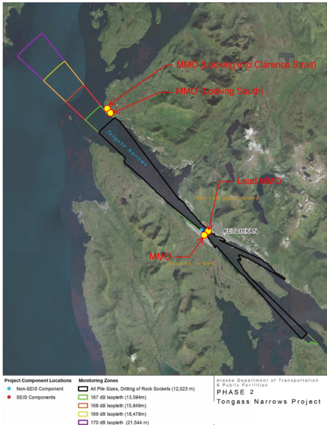
Figure 5.4: Marine Mammal Monitor locations during Revilla + Gravina simultaneous drilling/hammer work. One MMO on each rig; two MMOs at South Point Higgins, one looking into Tongass Narrows and the other Clarence Strait.
