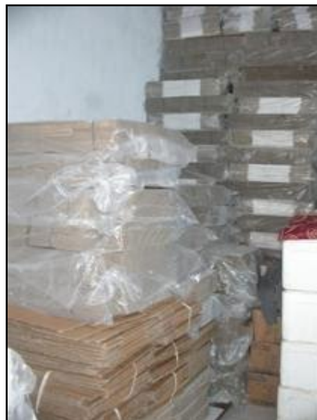
Insufficient space between the wall and packaging
