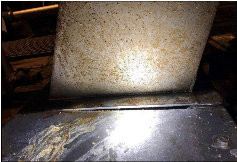
Gap observed in the protective cover of the auger
