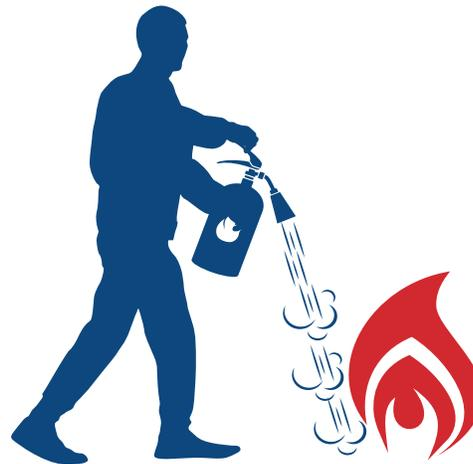
Discharge the fire extinguisher at the base of the fire.
