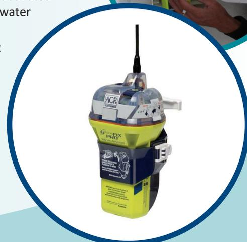
Top: EPIRB in hydrostatic housing.
