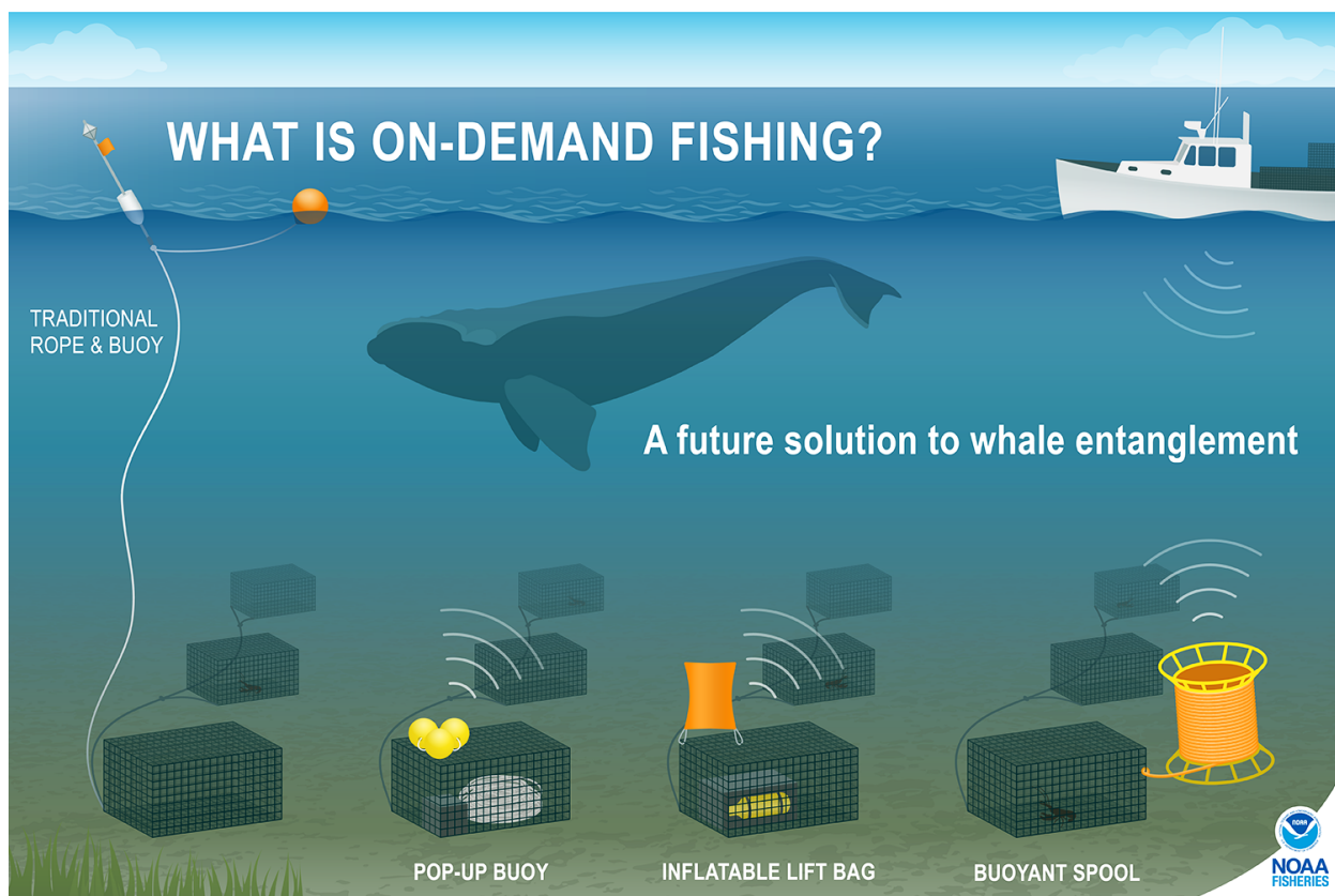
Figure 3. Fishing traps using a traditional lobster trap, lines, and buoys (left), and three on-demand fishing systems (right).
