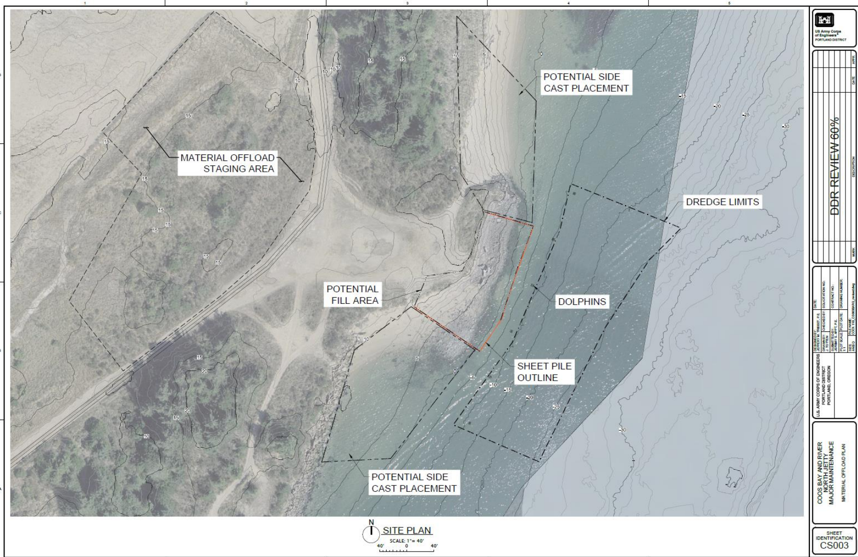
Figure 1-5. Material Offloading Facility Overview
