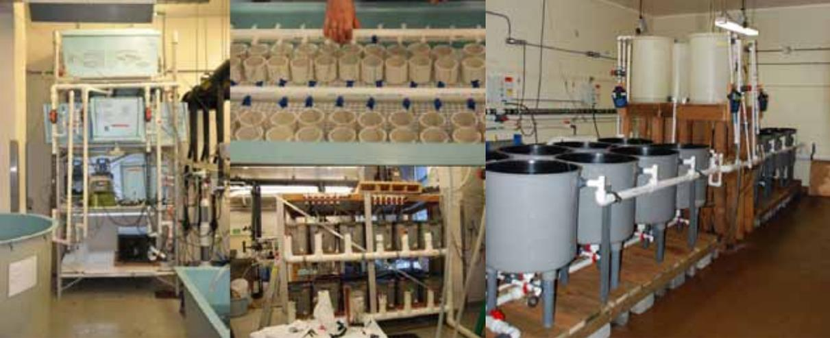
Figure 3. Experimental CO<sub>2</sub> dosing systems at the Kodiak and Newport Laboratories.
