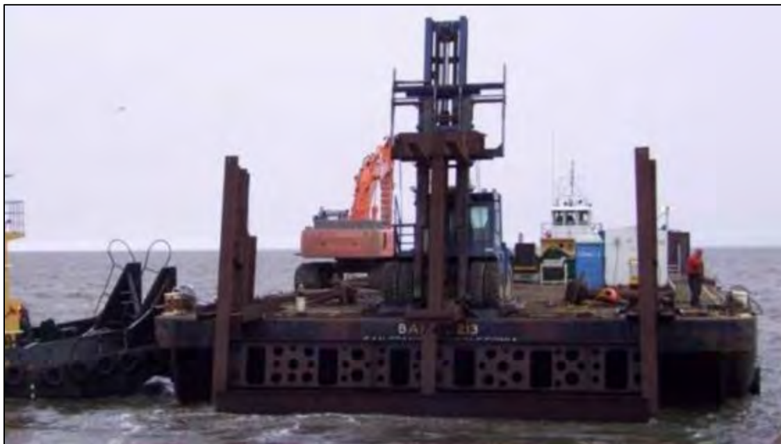
Figure 6: A Screeding Barge with the Screed Blade Raised
