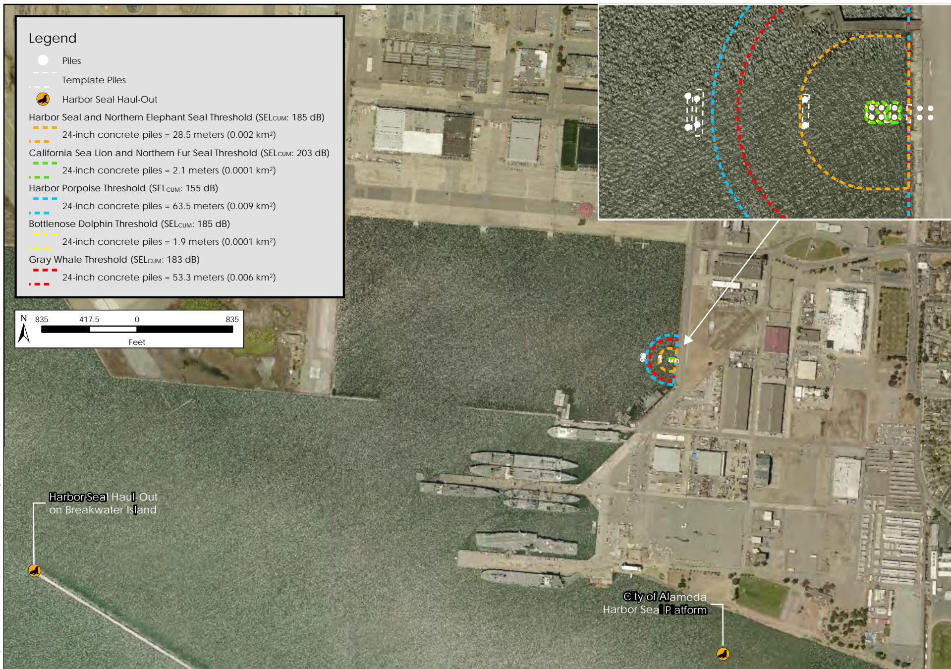
Figure 5. Distances to NMFS Level A Acoustic Thresholds for Impact Pile Driving
