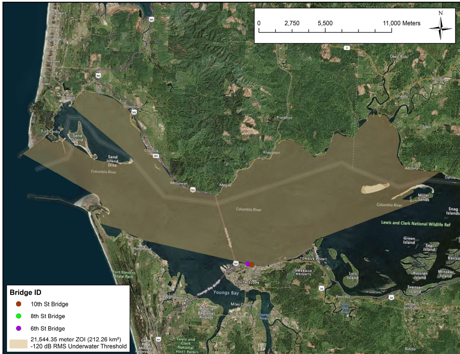
Figure 11 – 36-inch Temporary Casing Vibratory Install/Removal Level B ZOI
