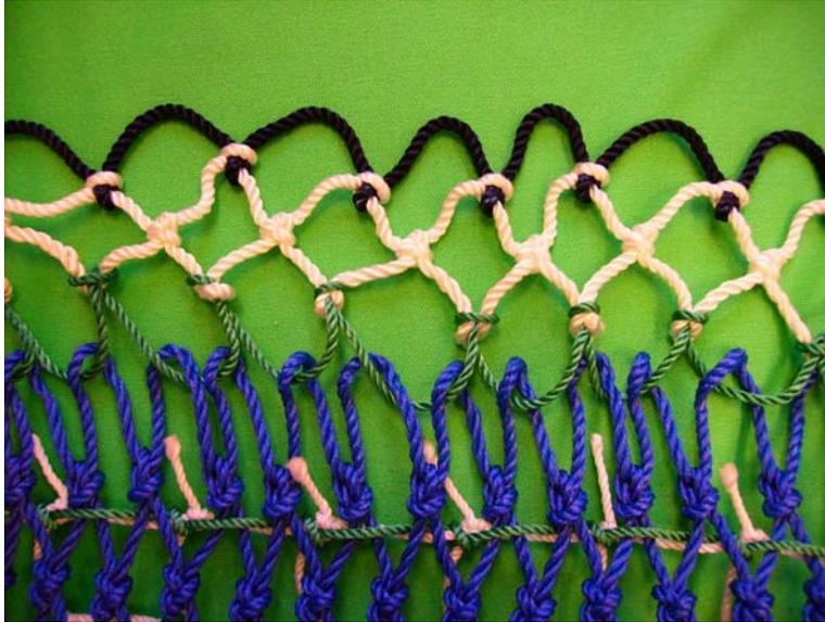
Figure 9: Attachment of the leading edge of the diamond mesh of the composite panel (blue) to the BRD extension (white).
