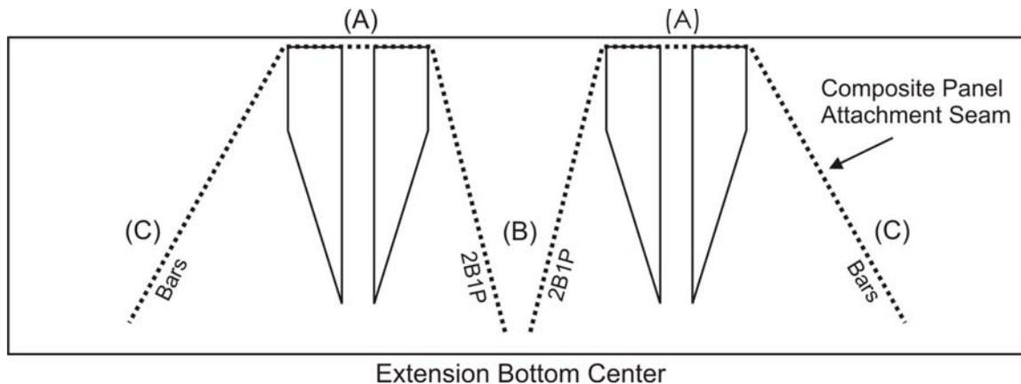
Figure 8: A schematic for the attachment of the composite panels to the BRD extension. (A) leading edge attachment, (B) inner seams, (C) outer seams
