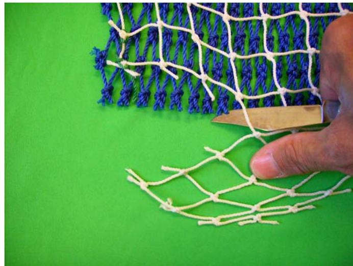
Figure 7: The end of the square mesh panel should be even with the last row of meshes on the diamond mesh. If the square mesh is too long, excess webbing should be cut off.
