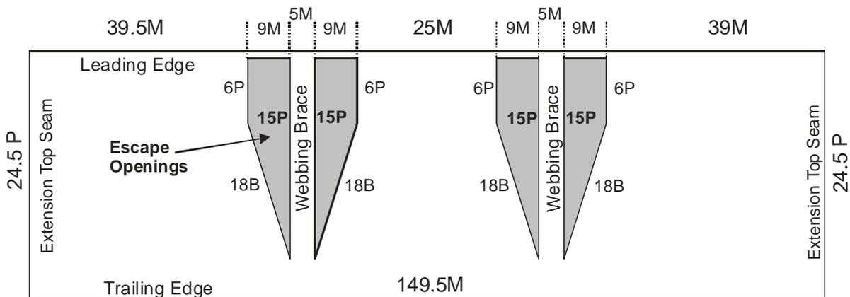
Figure 4: Schematic of BRD extension showing escape opening placement and configuration.
