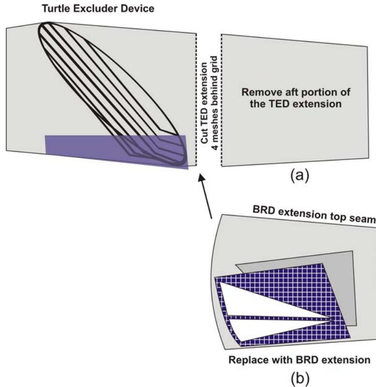
Figure 10: The Composite Panel BRD is installed in the trawl by removing a portion of the TED extension starting four (4) meshes behind the TED grid (a) and replacing it with the BRD extension. The codend is then attached to the trailing edge of the BRD extension (b).
