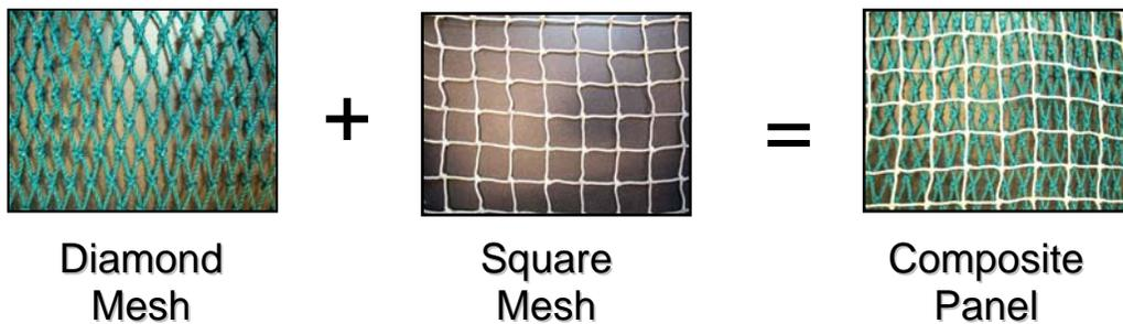
Figure 2: Components of the Composite Panel
