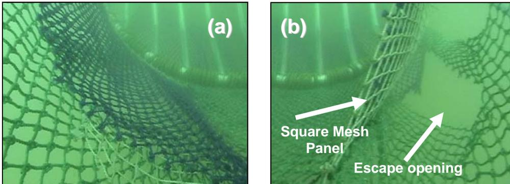
Figure 3: Composite panel on the port side with the square mesh component detached, causing the diamond mesh to collapse (a). Square mesh on the starboard side (b) supporting the diamond mesh maintaining space between the composite panel and trawl extension.
