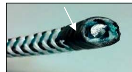
Leaded line showing lead core
