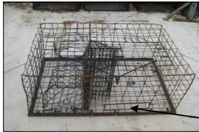
Rectangular escape port Highlighted for emphasis
