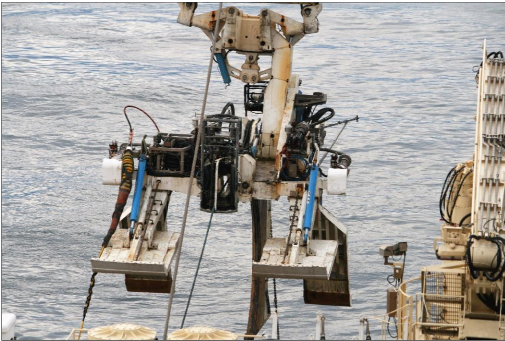
Figure 2-10. Sea Plow Being Hauled Aboard the Ile de Batz
