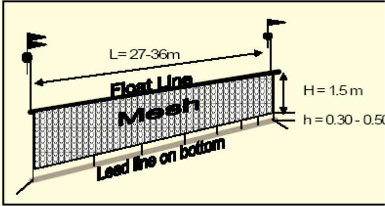
“Windows were created on the bottom of the net by adding nylon spacers 30 or 50 cm high. This allows the benthic sturgeon to slip through the net while the targeted species that swims slightly off the bottom will still get caught (Gessner and Arndt, 2006).
