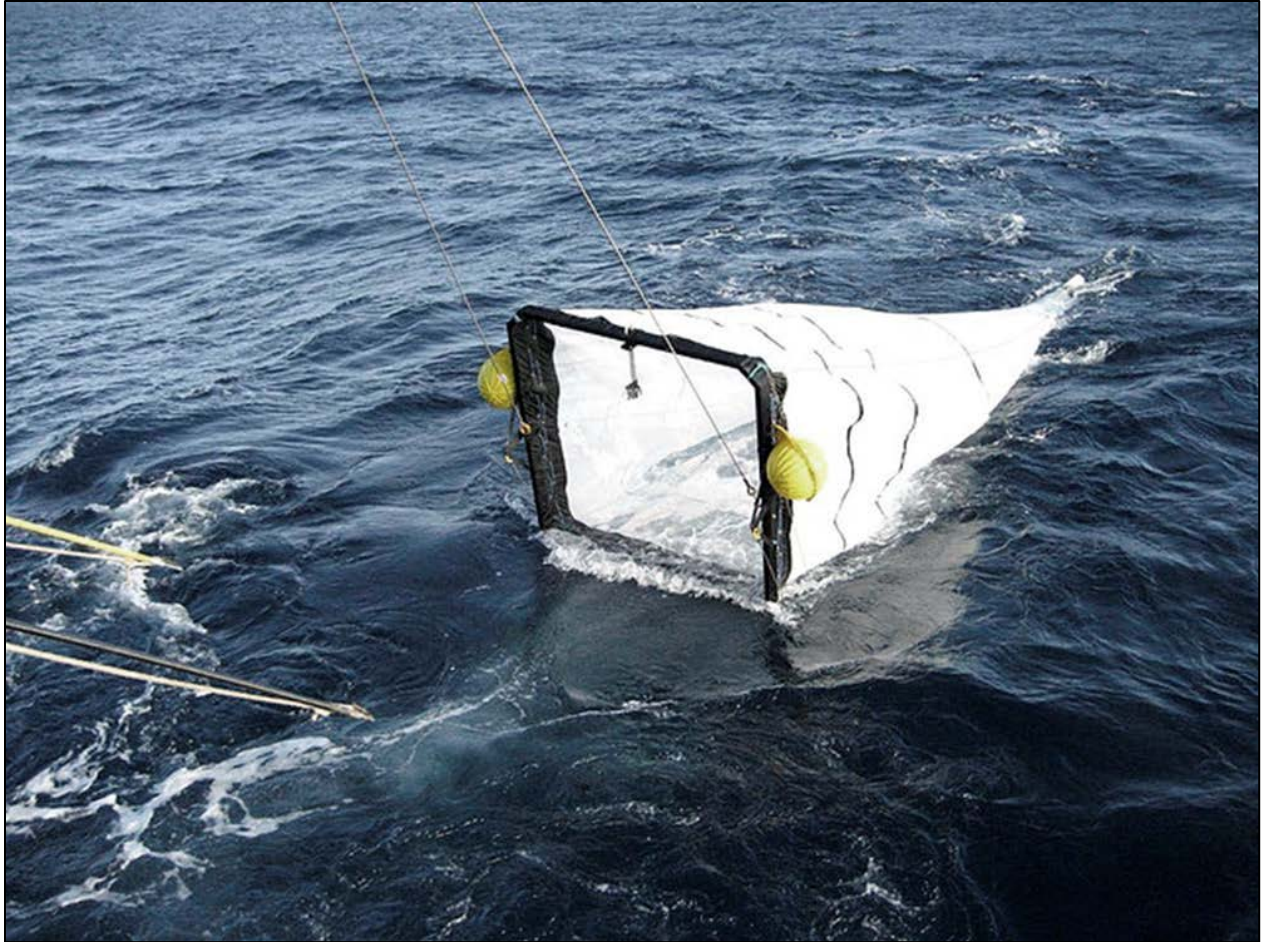
Figure B-2 Oozeki trawl at the surface as it is deployed from the vessel.
