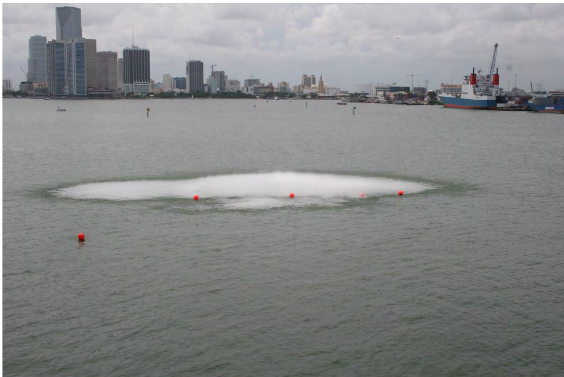
Figure 9 - Confined Blast of 1,361 kg (3,000 lbs) Total Charge Weight of Explosives
