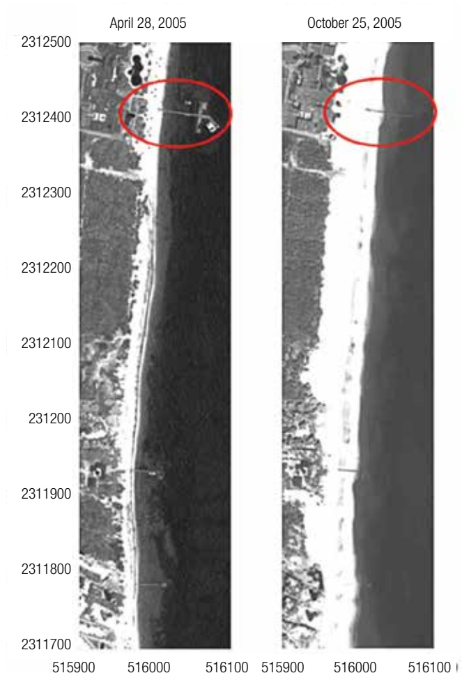
Figure 49. Effects of Hurricane Wilma in Puerto Morelos. Left, before and right after the hurricane. The beach was an accretion of almost 30 m across the coastline, also a large swath of vegetation was lost. One of the explanations, besides the sediment from Cancun, is that the last dune covered by vegetation was eroded and its sediment was redeployed on the beach profile (Mariño et al. 2014) (taken from Silva et al. 2014).
