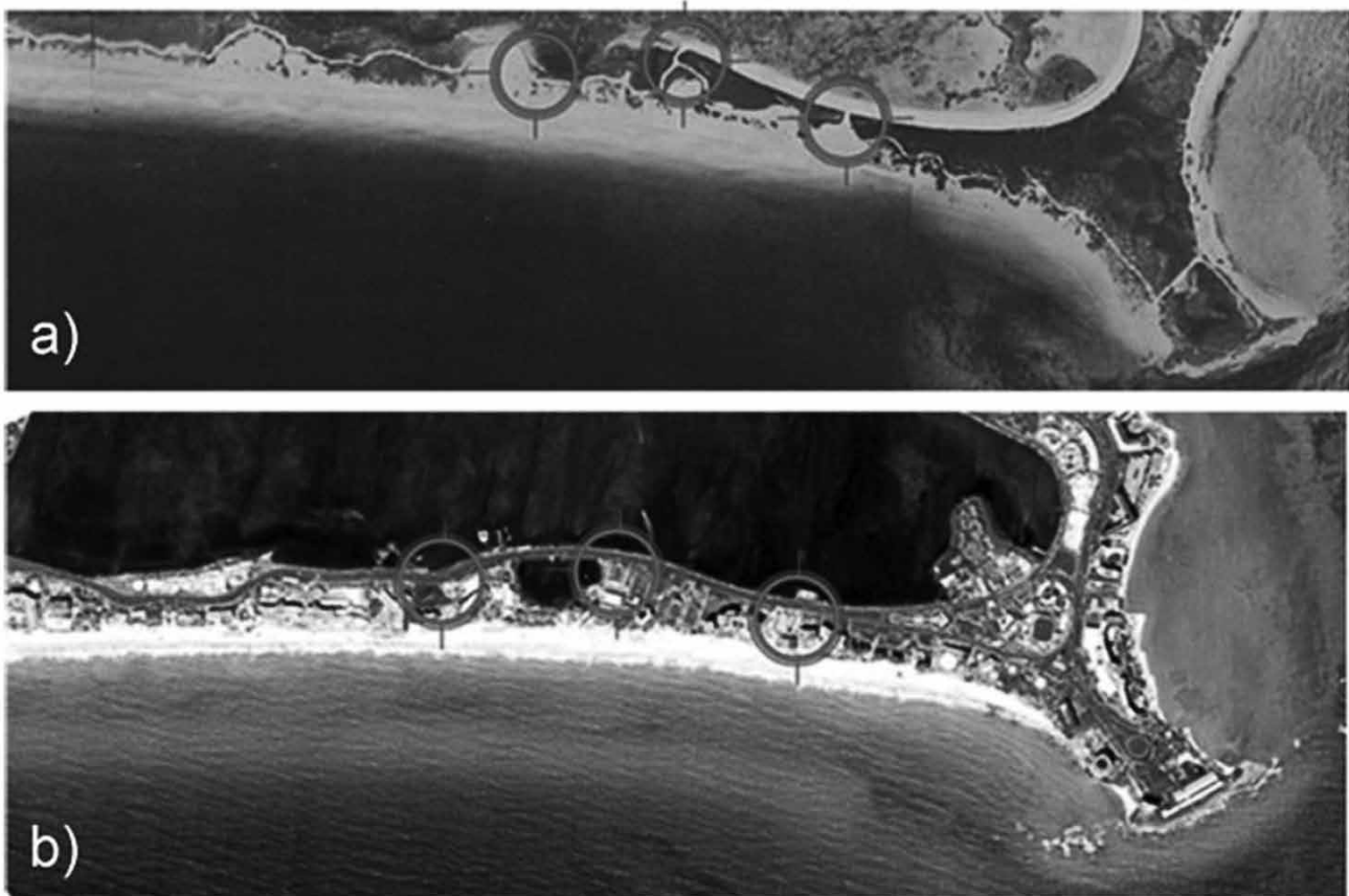
Figure 50. a) Punta Cancun in the 70's before the tourism development: The natural storm drains can be appreciated exposed during storm events. b) The current tourism infrastructure have modified and blocked storm drains (taken from Silva et al. 2012)
