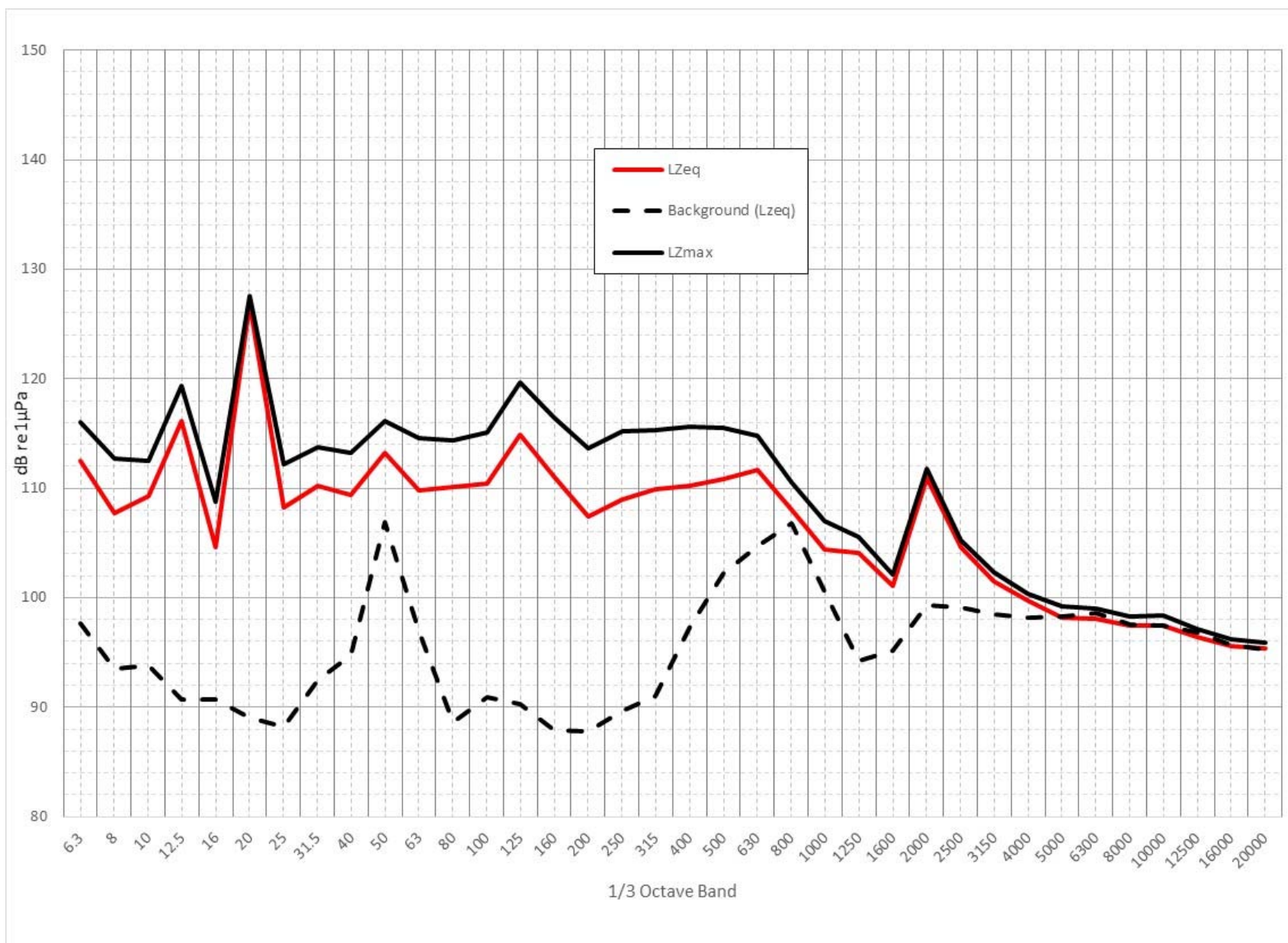
Figure B-2. 1/3 Octave Band Spectra for Installation of 24-inch Steel Shell Pile at 89 meters (292 Feet).
