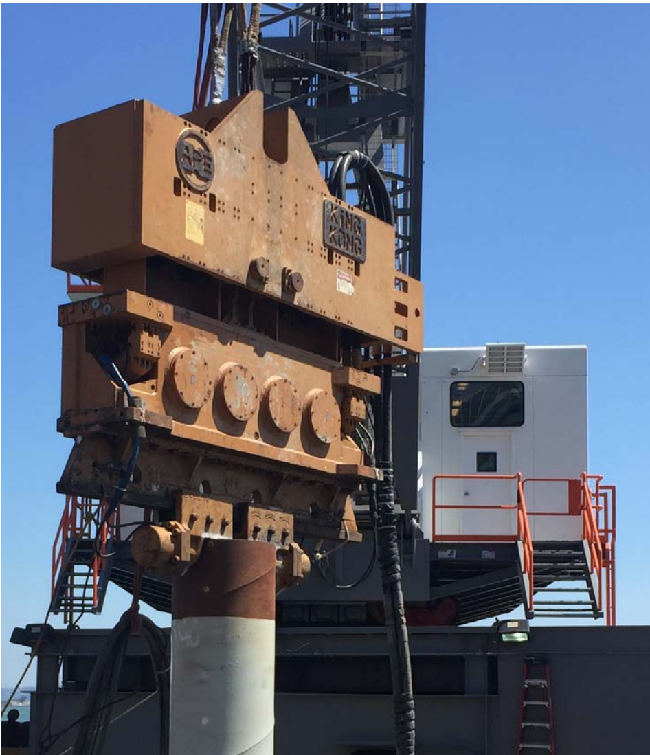
Figure 6. APE King Kong (Model 400P2) Vibratory Pile Driver
