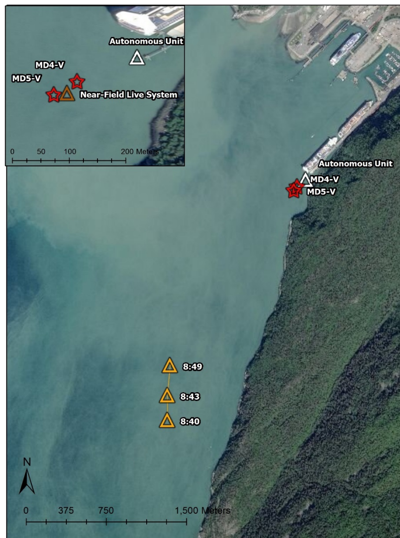
Figure 11. Rock socket drilling measurement locations in the far-field with an inset of near-field measurements on March 13 th , 2019. Far-field measurement locations ranged from 1.75 kilometers at 8:40 to 1.4 kilometers at 8:49 due to vessel drift.
