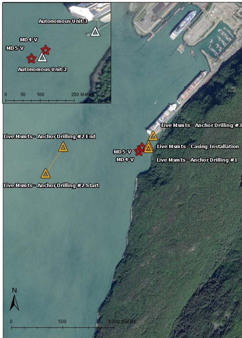
Figure 12. Rock anchor drilling measurement locations on April 13 th , 2019. Rock anchor drilling was measured at five positions ranging from 48 to 700 meters, while rock anchor casing installation was measured at one position of 30 meters. Two autonomous units were deployed in the near-field.
