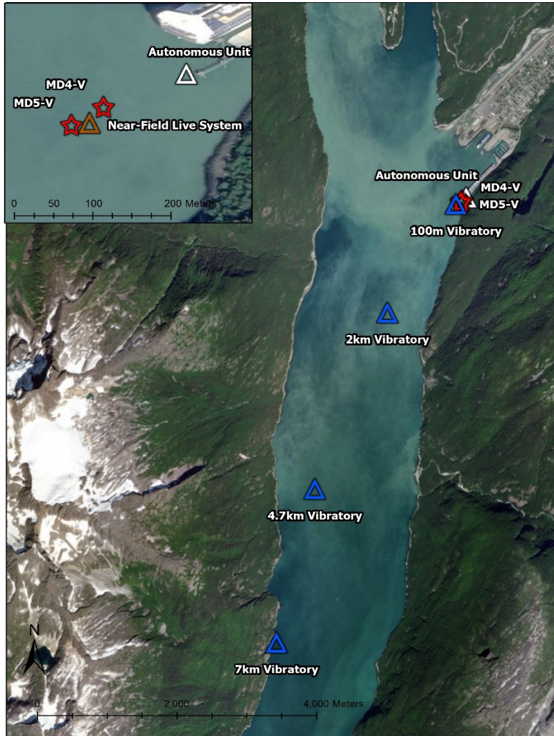
Figure 8. Vibratory pile driving measurement locations in the far-field with an inset of near-field measurements on March 8 th , 2019.
