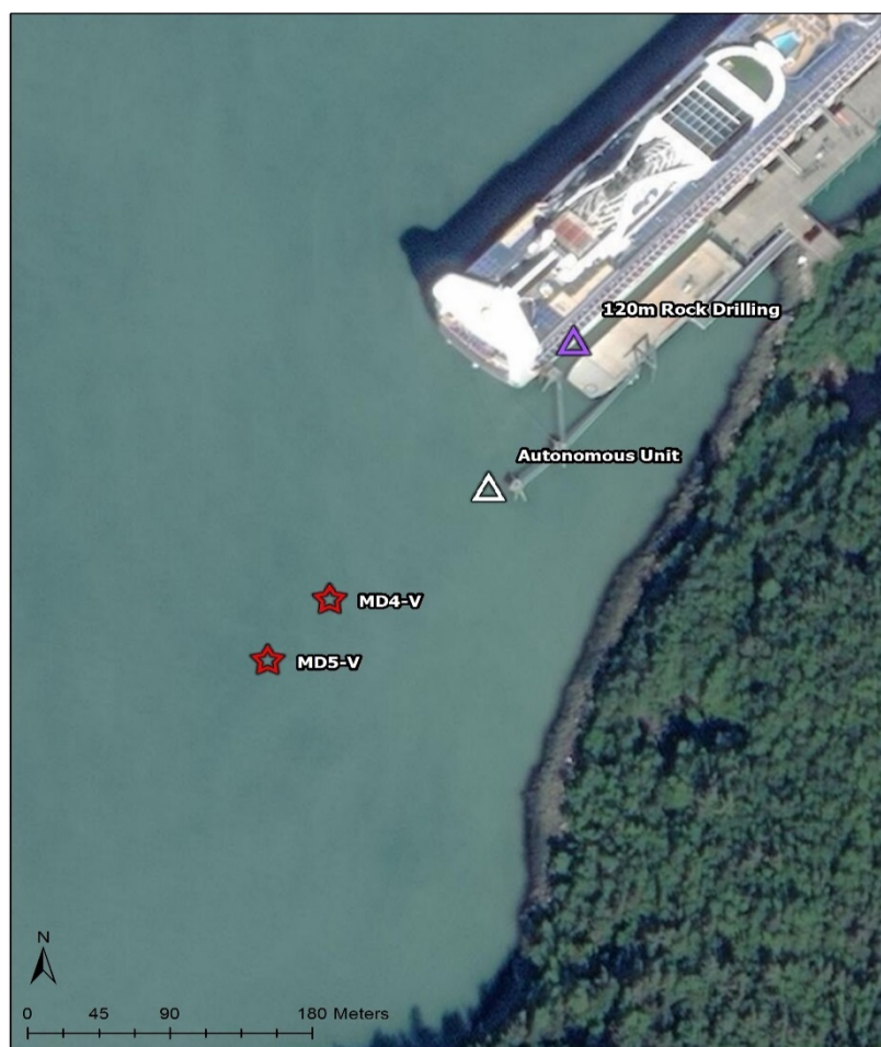
Figure 10. Rock socket drilling measurement locations on March 11 th , 2019. The far-field live system was deployed at 120 meters near the end of the docked barge and near-field live system measurements weren't taken on this date. Note that the distance of 120 meters was to the pile, while actual distances to the drilling sound source at the bottom of the pile was 128 meters from the shallow hydrophone and 122 meters from the deep hydrophone.
